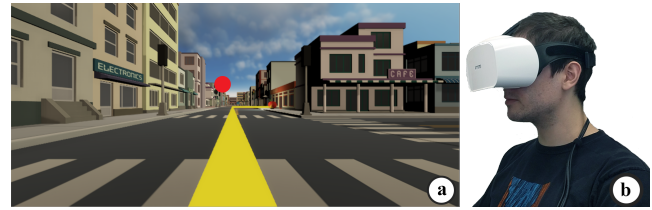
Figure 3: Participants of our data collection experiment completed missions while wearing the (b) FOVE eye-tracking virtual reality headset. Their position and gaze data were recorded and later used to train our LSTM. (a) The red dot—not shown to the participant during gameplay—depicts this participant’s gaze point, and the yellow navigation aid shows the closest path to the destination.
